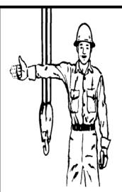
RAISE THE BOOM AND LOWER THE LOAD. With arm extended, thumb pointing up, flex fingers in and out as long as load movement is desired.
