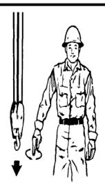
LOWER. With arm extended downward, forefinger pointing down, move hand in small horizontal circle.
