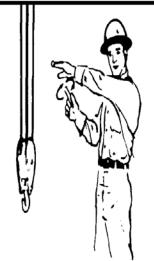
MOVE SLOWLY. Use one hand to give any motion signal and place other hand motionless in front of hand giving the motion signal. (Hoist slowly shown as example.)
