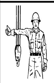
RAISE BOOM. Arm extended, fingers closed, thumb pointing upward.
