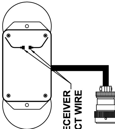
**NOTE: OPEN RECEIVER AND DISCONNECT WIRE**
