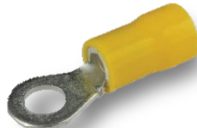
YEL RING INSUL P/N 16781 10-12GA #8 P/N 16111 10-12GA 0.25 P/N 15771 10-12GA 0.31 P/N 26725 14-16GA .437
