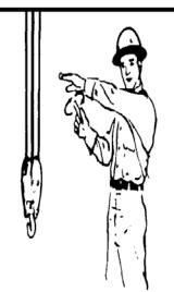
MOVE SLOWLY. Use one hand to give any motion signal and place other hand motionless in front of hand giving the motion signal. (Hoist slowly shown as example.)
