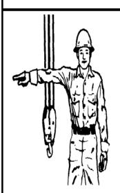
SWING. Arm extended, point with finger in direction of swing of boom.
