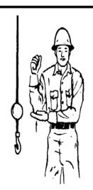
USE WHIPLINE (Auxiliary Hoist). Tap elbow with one hand; then use regular signals.
