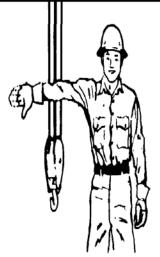
LOWER THE BOOM AND RAISE THE LOAD. With arm extended, thumb pointing down, flex fingers in and out as long as load movement is desired.
