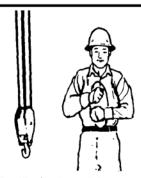
TRAVEL (Both Tracks). Use both fists in front of body, making a circular motion about each other, indicating direction of travel, forward or backward. (For land cranes only.)
