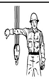
LOWER BOOM. Arm extended, fingers closed, thumb pointing downward.
