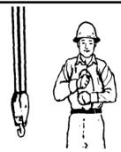
TRAVEL (Both Tracks). Use both fists in front of body, making a circular motion about each other, indicating direction of travel, forward or backward.
