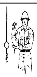
USE WHIPLINE (Auxiliary Hoist). Tap elbow with one hand; then use regular signals.
