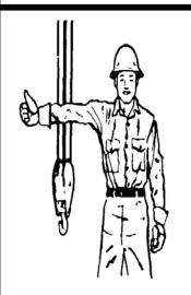
RAISE BOOM. Arm extended, fingers closed, thumb pointing upward.
