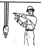
MOVE SLOWLY. Use one hand to give any motion signal and place other hand motionless in front of hand giving the motion signal. (Hoist slowly shown as example.)
