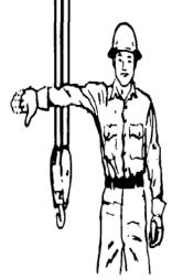
LOWER THE BOOM AND RAISE THE LOAD. With arm extended, thumb pointing down, flex fingers in and out as long as load movement is desired.
