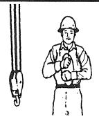
TRAVEL (Both Tracks). Use both fists in front of body, making a circular motion about each other, indicating direction of travel, forward or backward.
