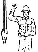
TRAVEL. (One Track) Lock the track on side indicated by raised fist. Travel opposite track in direction indicated by circular motion of other fist, rotated vertically in front of body. (For land cranes only.)
