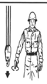
LOWER. With arm extended downward, forefinger pointing down, move hand in small horizontal circle.
