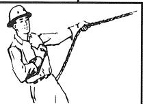
EXTEND BOOM (Telescoping Boom). One Hand Signal. One fist in front of chest with thumb tapping chest.
