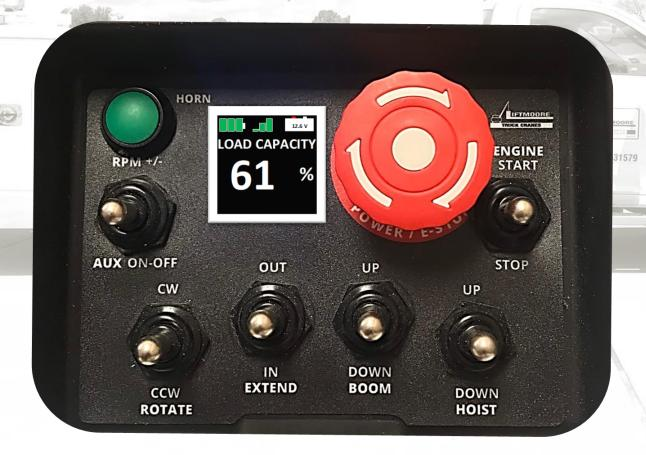
Liftmoore's Proportional Wireless Control for Electric Cranes with Diagnostics via On-Board WiFi
