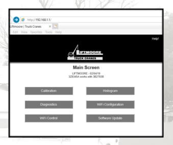
Also included in the menu options is a Histogram page, which indicates any active errors and the number of times an error or fault has been recorded for the life of the control system
